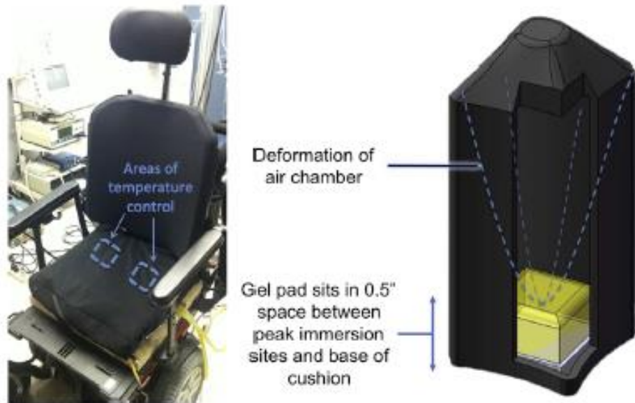
Fig. 1. Prototype temperature control wheelchair seat cushion. (Left) Blue squares indicated areas of temperature control for the left or right ischium. (Right) Cushioning cooling element were added to 4 air cells beneath each ischium location. (For interpretation of the references to colour in this figure legend, the reader is referred to the Web version of this article.)
